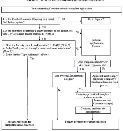
Figure 1 – Inverter Based Simplified Interconnection Process
