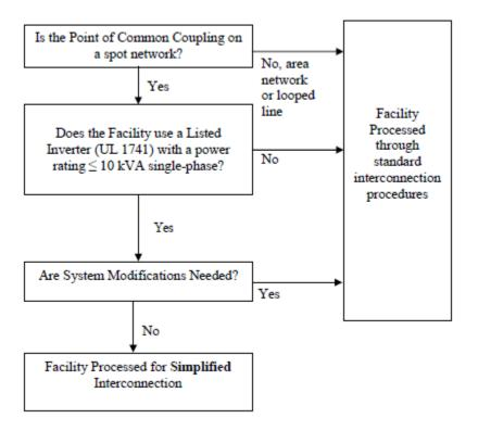
Figure 2 - Simplified Interconnection to Networks
